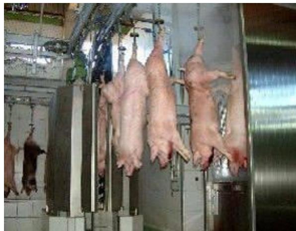
**SCALD VERTICALLY:** *The animal is scalded by means of warm, but this water is distributed across a few diffusers placed along the tour in different heights, in order which the animals are scalded homogeneously throughout the time of permanency inside the machine. All the controls and levels are controlled automatically, by means of electronic programmers.*
