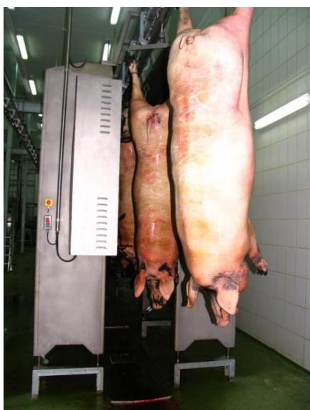
A vital complement for these lines is the oven chamuscador, which stays the remains of hair once spent the animal for the first flageladora of dried. Our oven can work both with propane and with natural gas, and is prepared in order that the columnas work only where the animal happens. An ideal complement is to use the second oven as descontaminador at the end of the line.
