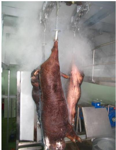
*One of the most important tasks inside the process of slaughter is the cautious one, since it is fundamental to realize a good process of depilated. For it A.M.S MEAT SYSTEM, account with the most rigorous systems of control of temperature, and developing for our clients three systems of scalded:*
