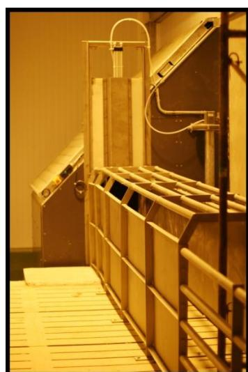
**CO<sub>2</sub>:** His bewildered one is by means of gas carbon dioxide, which is in a pit. The animals are introduced in a few cages which go down up to the pit across a system of chain driven electrically. The cage realizes a cycle remaining inside the pit the necessary time in order that the animal finishes slept. Depending on the production they will place more or less jaulas.
